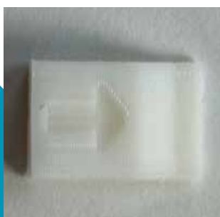
MicroSD card pusher Tool for Mechanical Alignment
