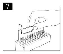
After the Comb has completed the cycle for **Row F**, transfer it back to **Row E**. Incubate in **Row E** for **2 minutes** for color fixation.
