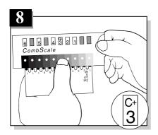
**A**. When the Comb is completely dry, align it with the calibrated color CombScale provided in the kit. Find the tone of the purple-grey on the CombScale that most closely matches the **Positive Control spot**. Slide the yellow ruler until the C+ mark appears in the window above the color you have found. **Hold the ruler in this position during the entire reading.** This step actually calibrates the C+ to S3, which is the "cutoff" point to which test spots will be compared.
