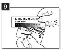
**B.** While holding the ruler, find the tone of purple-grey on the CombScale that most closely matches the desired **test result spot** (one of the lower spots). The number that appears in the window above is the CombScale score (S0-S6).
