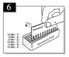
Pierce the cover of wells in **Row B** with the tweezers. Gently shake off excess liquid from the Comb onto a tissue (follow the same procedure for remaining rows at the end of each step). Insert Comb into wells of **Row B** and incubate for **2 minutes**, shake off and transfer the Comb to **Row C** and incubate for **10 minutes**. Place the Comb in **Row D** for **2 minutes**, **Row E** for **2 minutes**, and **Row F** for **10 minutes**, allowing the color reaction process to develop.
