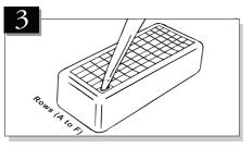
Dispense sample into each well. When using capillary tubes raise and lower the piston several times to achieve mixing. When using a pipette, mix by depressing the plunger a number of times.
