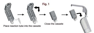
Place reaction tube into the device
